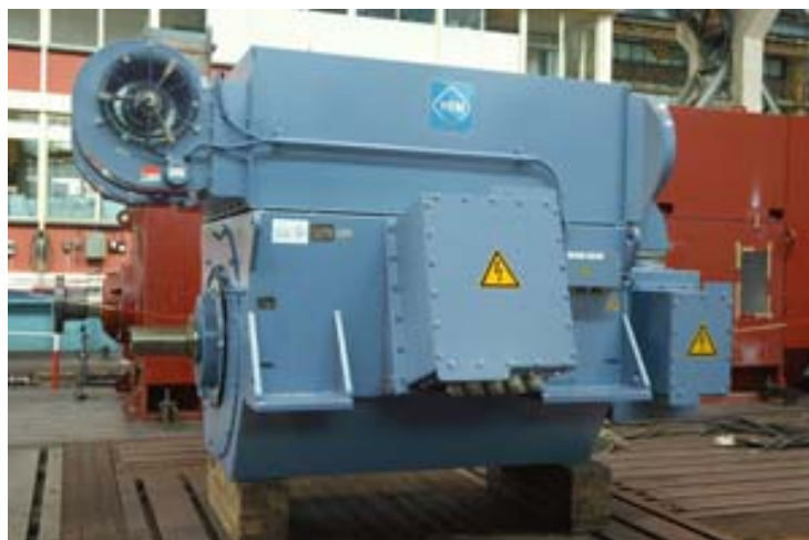
Fig. 6.21. Generator electric eolian de 5MW
