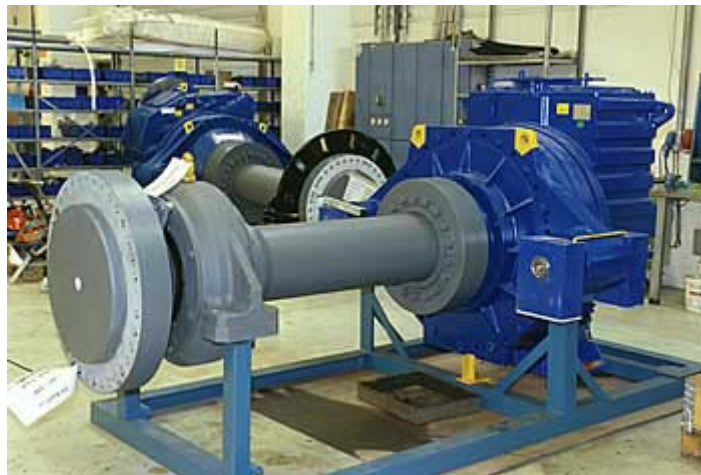
Fig. 6.15. Arborele principal al unei turbine eoliene www.windpower.org
